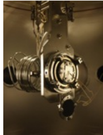
Figure 1: Six-axes goniometer compatible with ultra-high vacuum with heating and cooling capabilities for investigations on collisions
